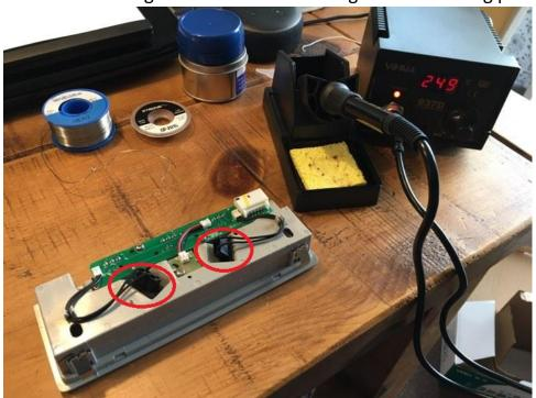
8. After a couple of attempts to directly solder my extension wires to the front pins powering the LED cabin lights, I gave up so instead I decided to bare the two black wires on each side that feed the cabin LED's and solder my extension cables.
