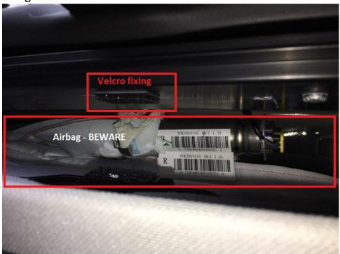
18. Use Stanley knife to cut around the pencil mark but ensure you do this with your hand inside the roof liner whilst you pull the liner down and away from the airbag. The roof liner is made of foam, so it is easy to cut through.
