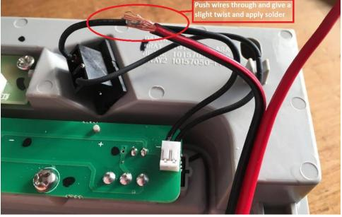
9. Bare all 4 black cables (both pairs at each side) and follow the same process of pushing wires through and then solder and cover using
