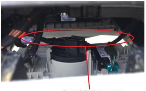
Gap in to cabin that you can use to feed electrical cables through.
