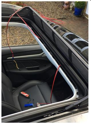
14. Next step was to expose the grab handle 8mm bolts using a fine flat head screwdriver. I loosened the bolts, but before pulling the handles free from the roof liner I offered up my crude rear light paper template. When I was happy with the position of the template, I used a pencil to mark out the roof liner cut line.
