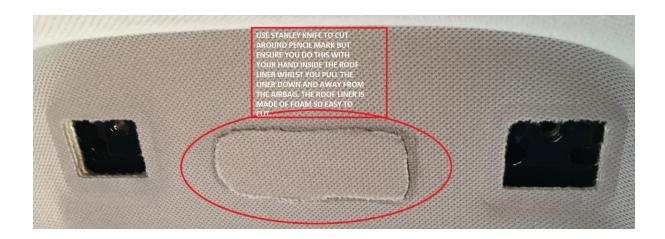
19. Remove roof liner foam. It might help if you slide your hand between rubber seal and roof liner to push excess foam out and repeat on other side.
