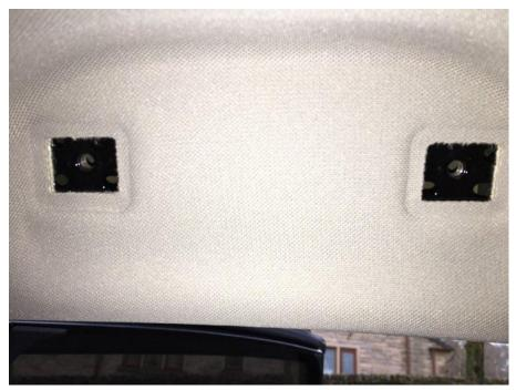
17. Now pull the roof liner in a downward motion to free this from Velcro fixings.
