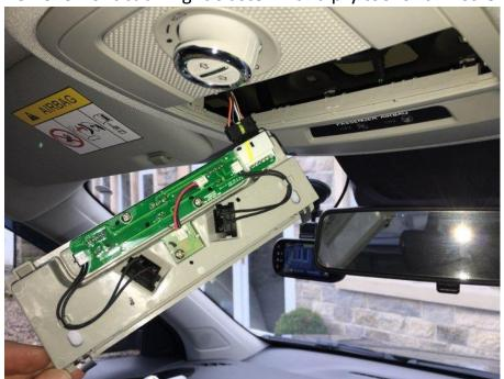
2. You will need to get a fine screwdriver and press the black stopper on the main connector to release this.
