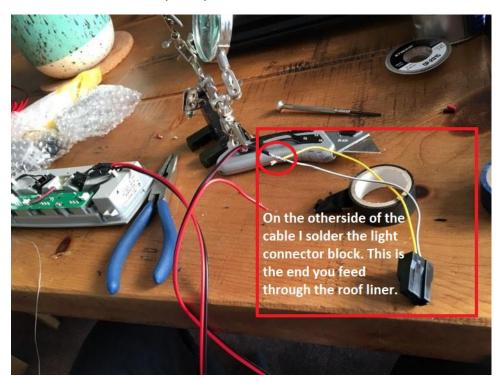
12. I also put additional electrical tape to join each of the wires and to tidy these up.
