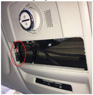
4. Open sky roof. At this point I sat on centre arm rest with head sticking out of sky roof and pulled down on the roof liner which is held in place by strong Velcro and clips to create a gap to feed the wires through.
