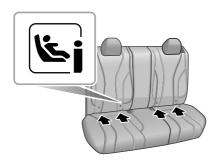
3 To fasten the Top tether strap of the child restraint system, route the tether strap under the head restraint and attach to the anchorage hook being careful not to twist the strap. If not using ISOFIX lower anchorages, using the seatbelt, complete the installation in line with the child restraint manufactures instructions.
