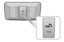
The emergency services call (eCall) system will perform a self-test when the vehicle power system is ON. During a Self-Test the emergency services call (eCall) LED status indicator on the SOS button will flash quickly until completion. The LED status indicator will be illuminated solid if no system faults are present. The LED status indicator will not illuminate or flash slowly if a fault is
