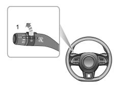
With the START/STOP Switch in the ON/READY position and the headlamps on, rotate the fog lamp switch to position I to turn on the rear fog lamps. The rear fog lamp
